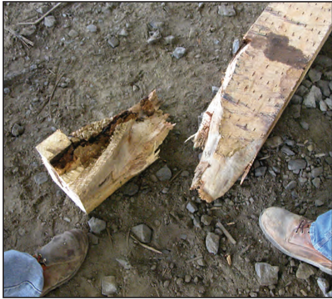
Figure 36. A crossgrain problem with this tie was caught before treatment—it broke when it was dropped!
