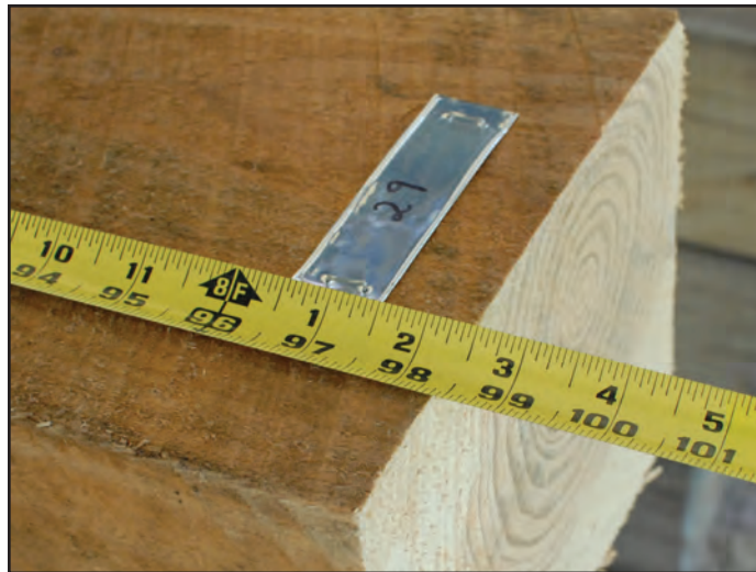
Figure 13. An example of a short pine tie that made it to a treatment plant. It should have been 8' 6" (102") long.
