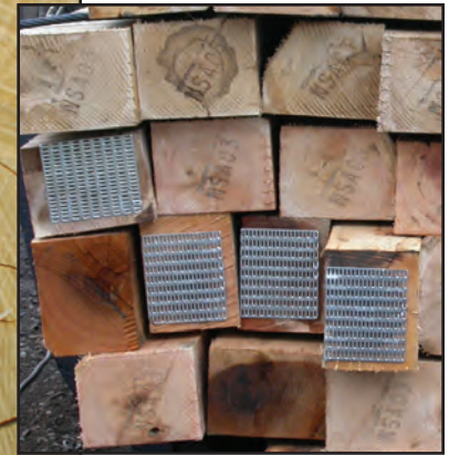
Figure 7. Some of these ties have been end-plated.
