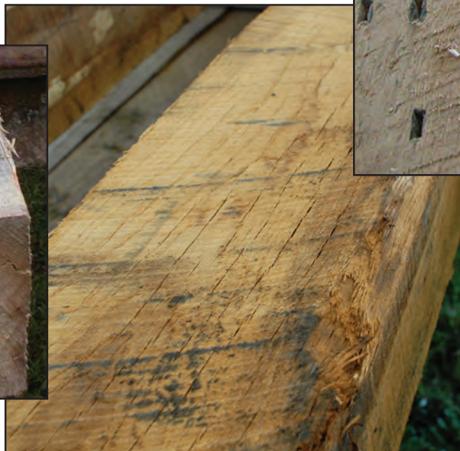
Figure 5. Mechanically incised tie.
