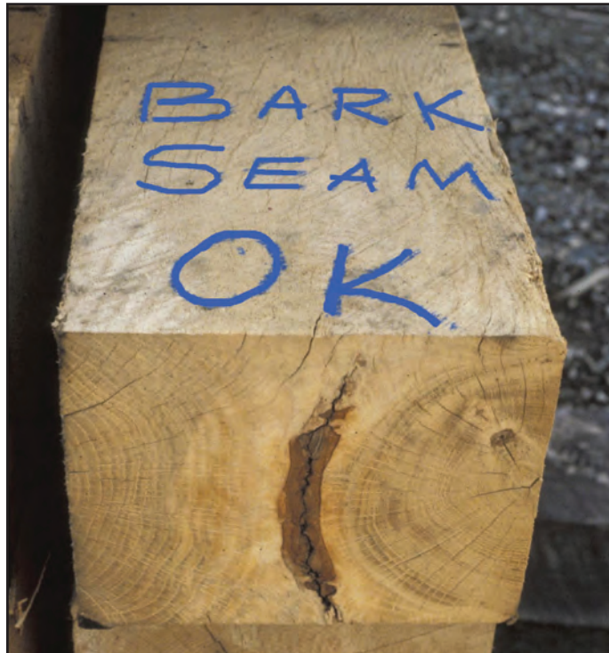
Figure 32. A bark seam that would probably be acceptable.
