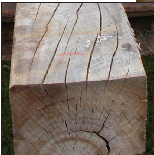
Figures 3 and 4. Compare the checking patterns on the sweet gum crosstie (above) to the white oak tie (right).
