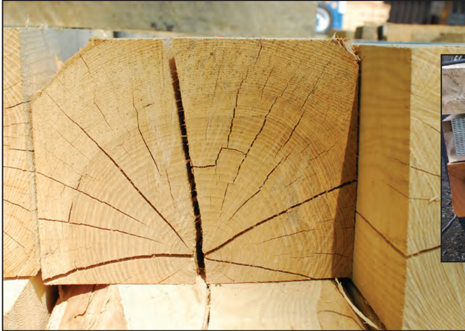
Figure 6. A platable split in an ash tie.
