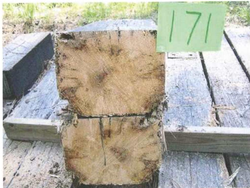
**Figure 36** - Tie #171 (red oak/control) with decay visible in cross-section.
