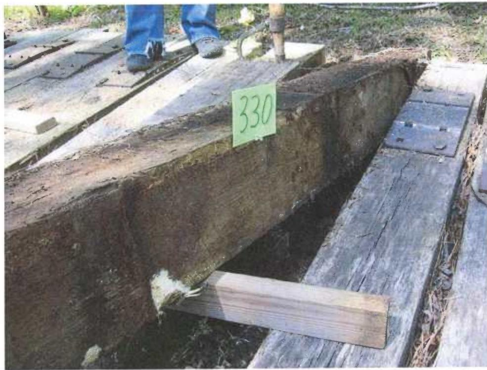
**Figure 61** - Tie #330 (Envirosafe/white oak) with termite grazing and trace decay.
