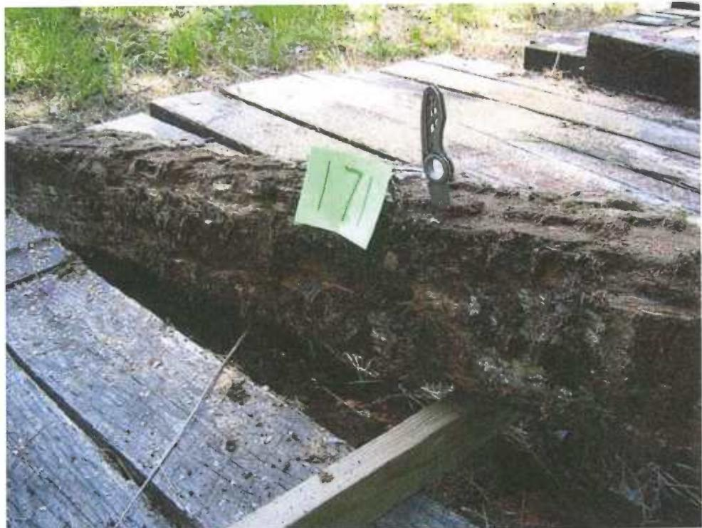
**Figure 35** - Tie #171 (red oak/control) with heavy decay on bottom.
