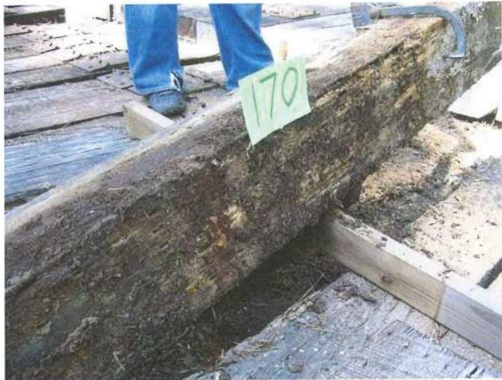
**Figure 33** – Tie #170 (white oak/control) with slight decay on bottom.
