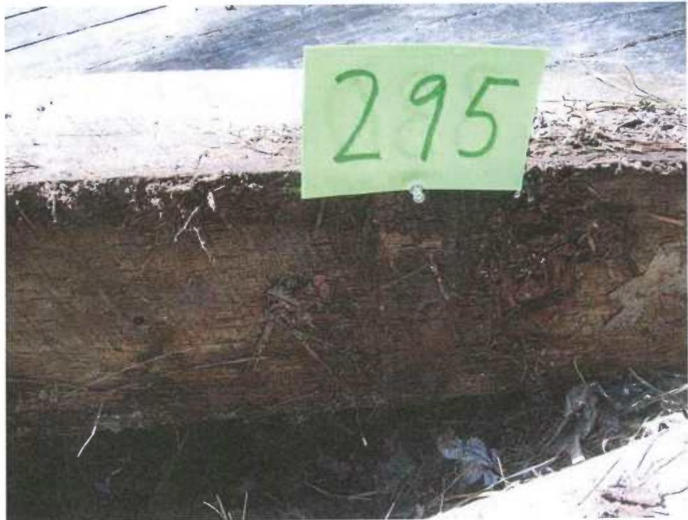
**Figure 59** - Tie #295 (Envirosafe/red oak) with live termites (surface etching) and trace decay.
