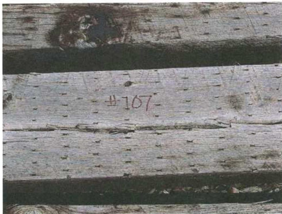
**Figure 6** - Tie #107 (Nisus) with checking.
