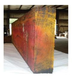
Fig. 7 White Oak Cross Section Boron Rod Diffusion
