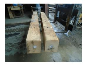
Fig. 1 Boron Rod Drilling Pattern with Plugs
