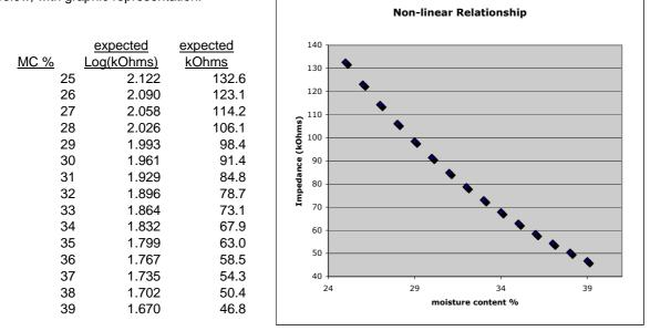
Average moisture content from a sample of ties can produce results which are biased in terms of targeting an expected value of impedance. For example, two ties with MC of 25 and 39 have an average MC of 32. The expected impedance, according to the equation, is 78.7. However, the true impedance values are 132.6 and 46.8, with an average impedance of 89.7, which is almost 14 percent higher than the "true" average value.
