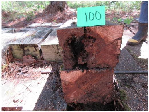
**A20** – Tie #100 (Lonza/red oak) significant internal deterioration.
