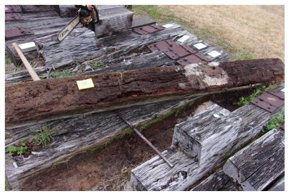
A81 - Tie #88 (Lonza/red oak) decay and termite damage on bottom.
