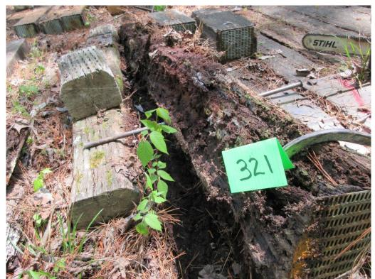
A45 - Tie #321 (untreated/white oak) with extensive decay and moderate termite damage.
