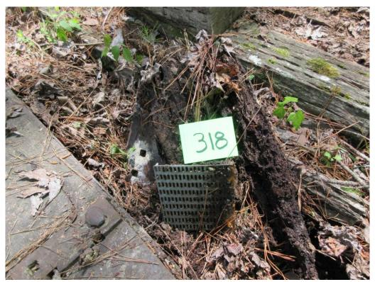
**A29** - Tie #318 (untreated/red oak) completely deteriorated.
