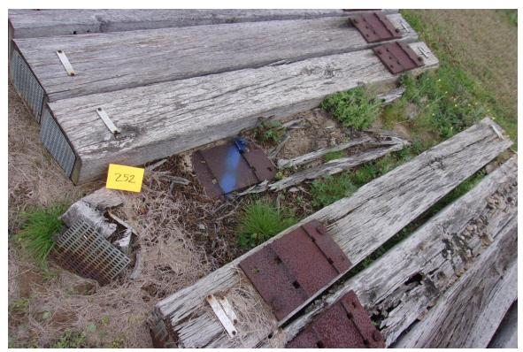
A97 - Tie #252 (untreated/red oak) failed due to decay
