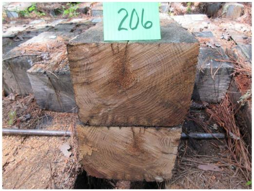
A42 - Tie #206 (Nisus/white oak/borate) with decay near checks & on bottom.
