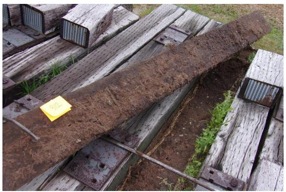
**A125** - Tie #312 (Koppers/white oak/creosote petroleum solution) with light decay & Formosan termite damage.
