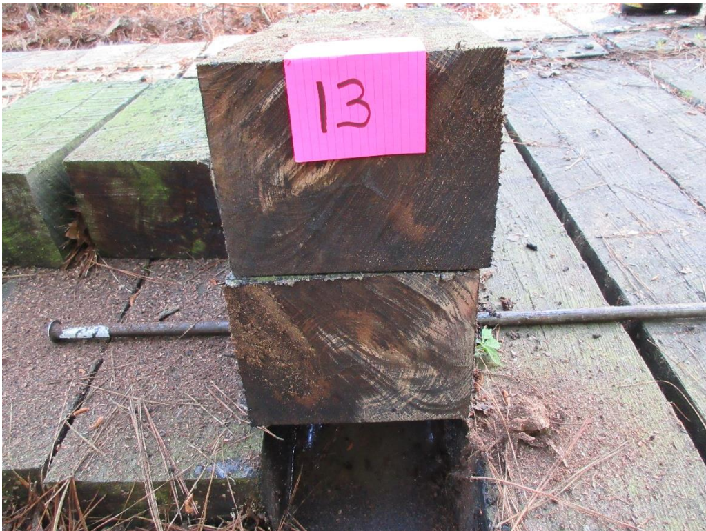
Figure 4 - Tie #13 red oak/borate/creosote 7lbs (Koppers).
