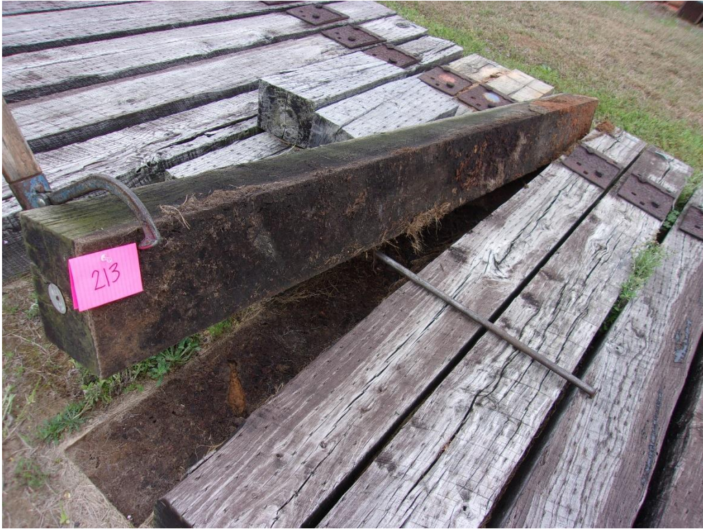
Figure 97 – Tie #213 red oak/borate/creosote 7lbs (Koppers).
