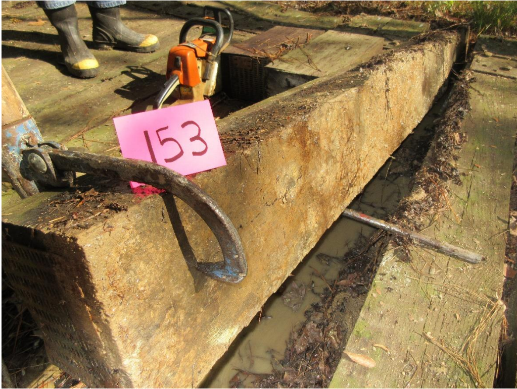
Figure 33 - Tie # 153 red oak/DOT/ACZA/oil (Lonza).
