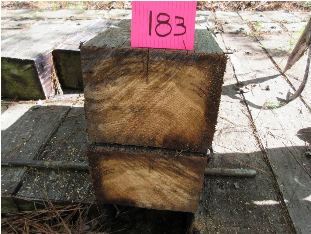
Figure 40 - Tie #183 Douglas fir/P2 creosote (Lonza).
