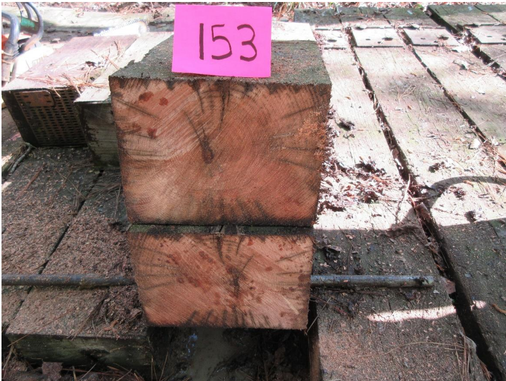
Figure 34 - Tie # 153 red oak/DOT/ACZA/oil (Lonza).
