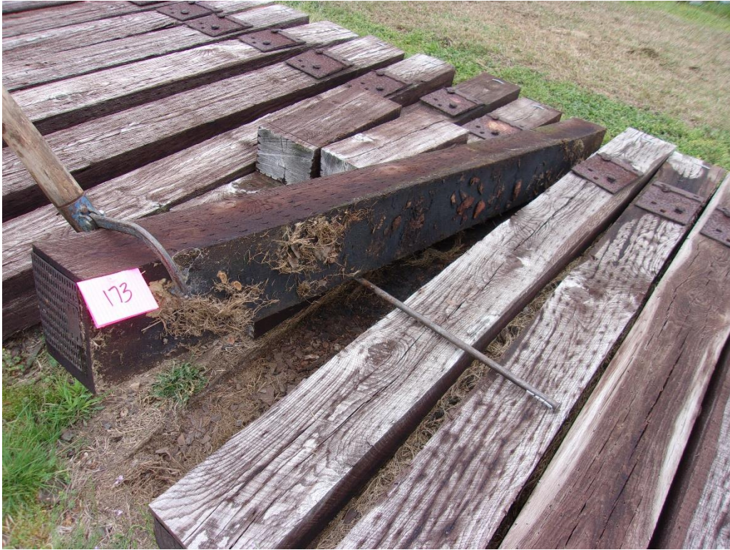
Figure 89 – Tie #173 white oak/DOT/ACZA/oil (Lonza).
