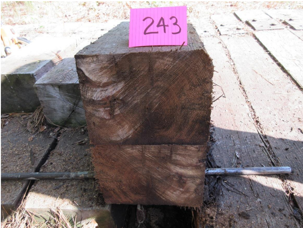
Figure 52 - Tie #243 red oak/ACZA/DOT/ET (Lonza).
