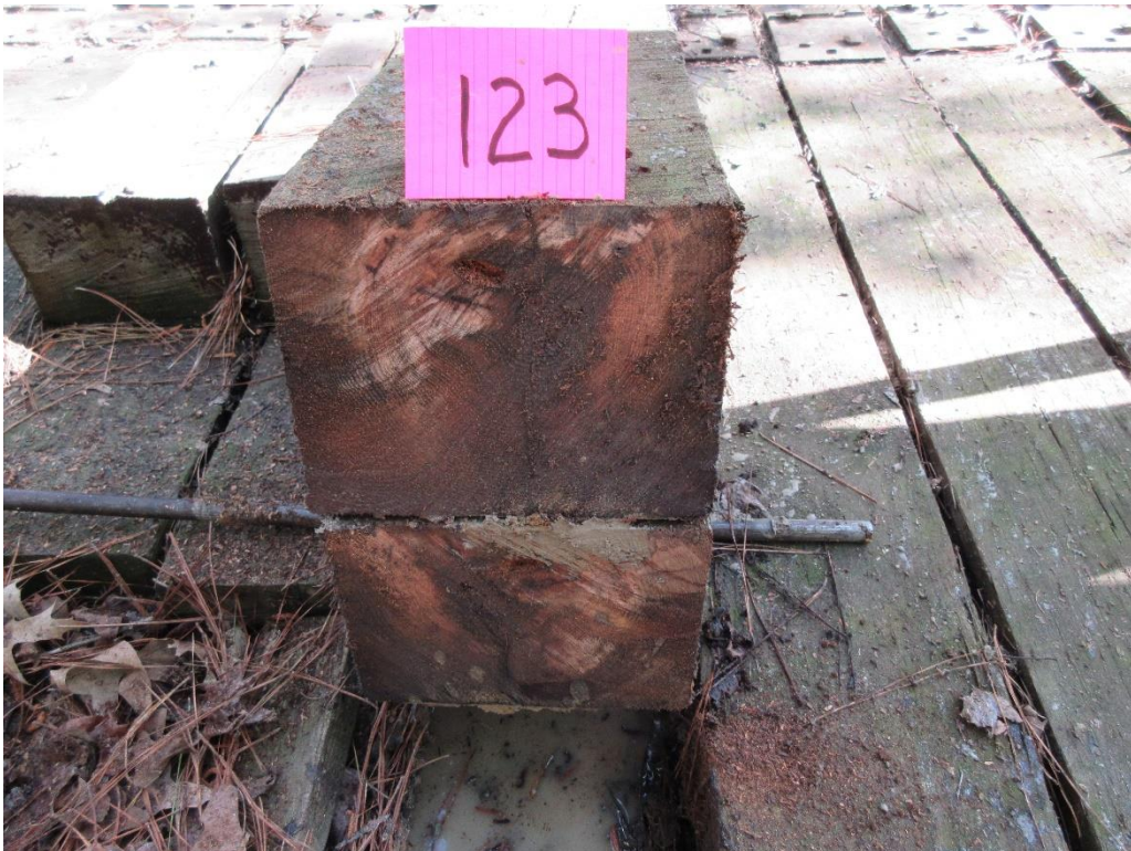
Figure 26 - Tie #123 red oak/DOT/ACZA/oil (Lonza).
