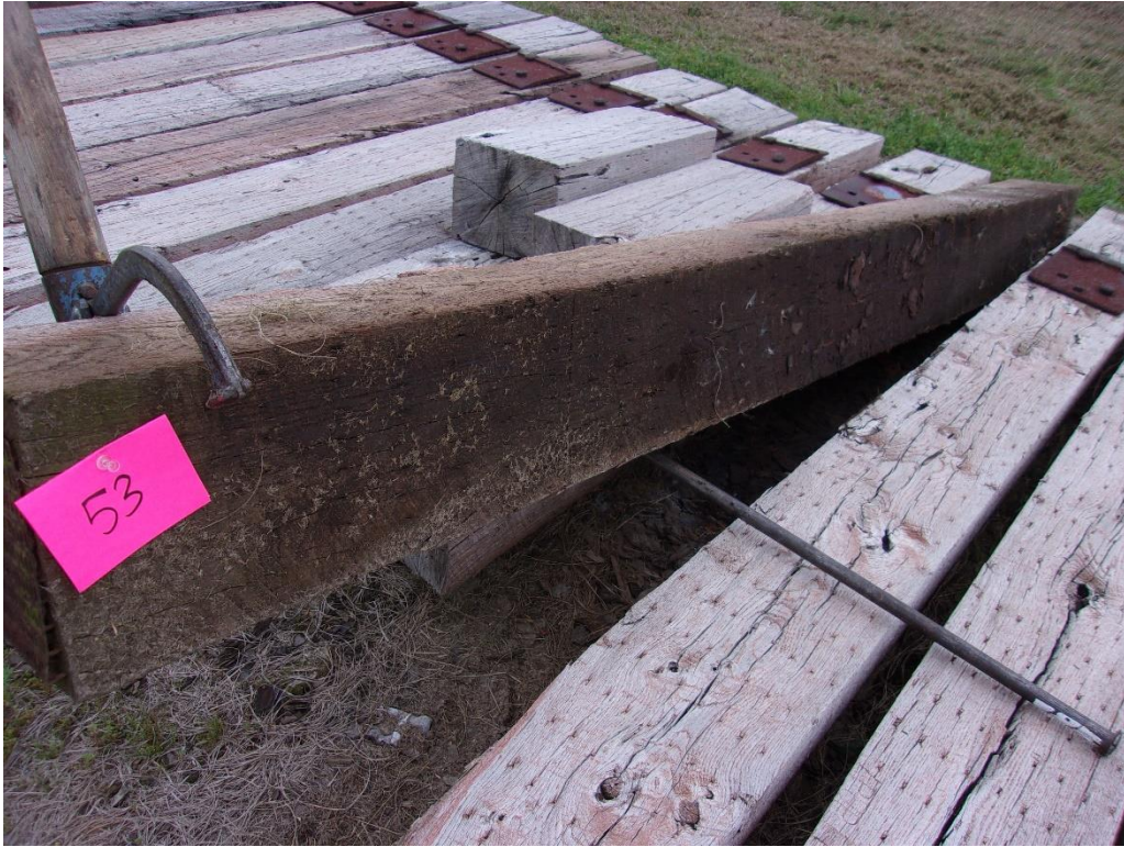
Figure 63 – Tie #53 red oak/DOT/ACZA/ET (Lonza).
