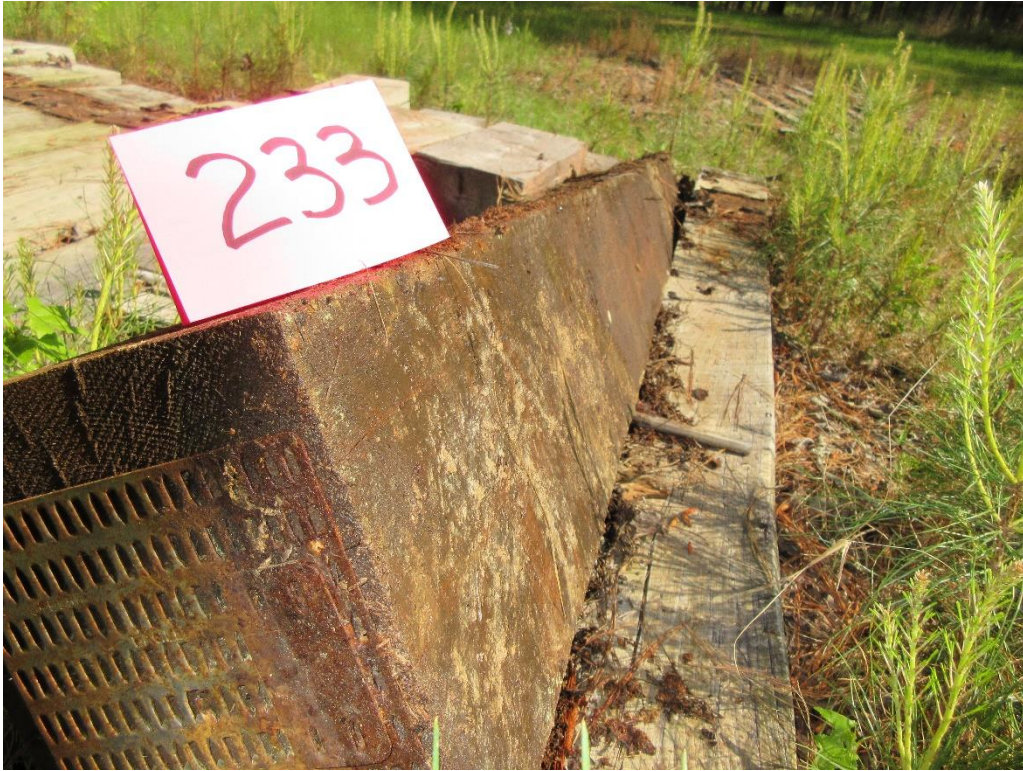
Figure 49 – Tie # 233 white oak/DOT/ACZA/ET (Lonza).
