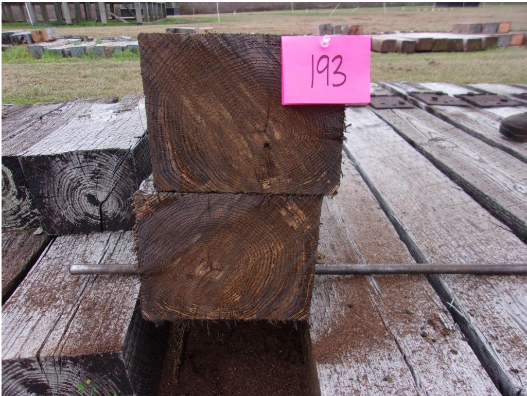
Figure 94 - Tie #193 white oak/borate/creosote 6lbs (Koppers).
