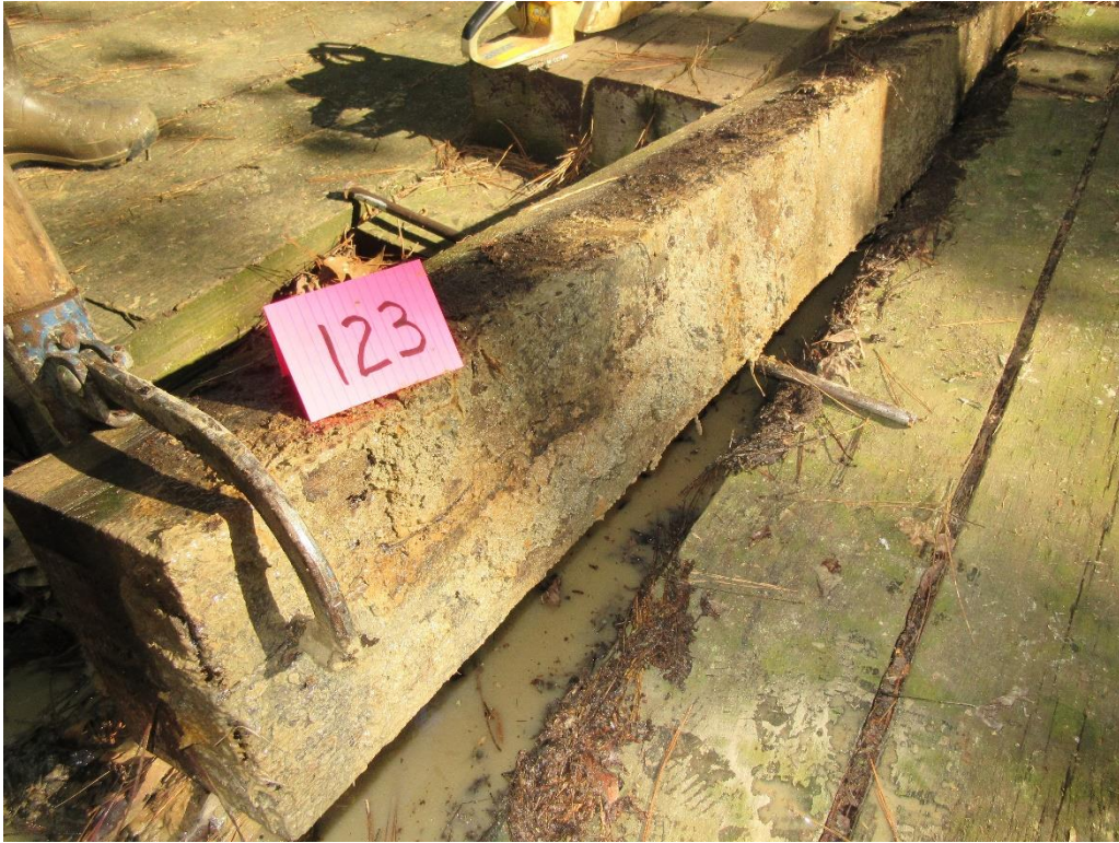
Figure 25 – Tie #123 red oak/DOT/ACZA/oil (Lonza).
