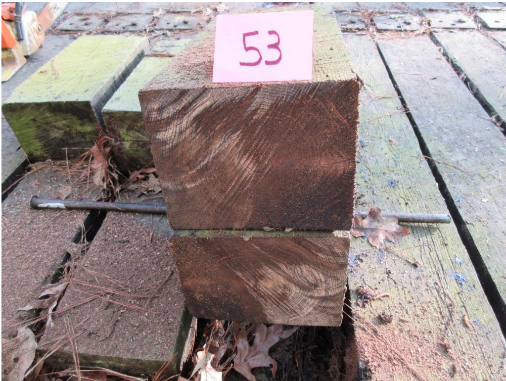
Figure 12 - Tie #53 red oak/borate/creosote 6lbs (Koppers).
