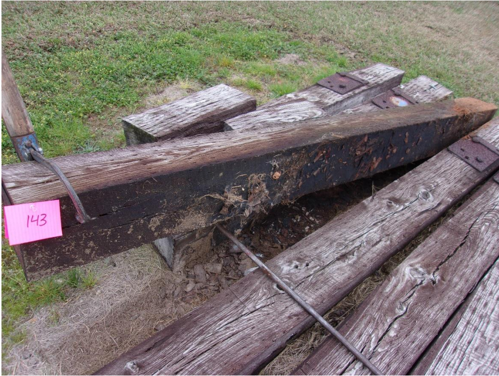
Figure 81 – Tie #143 red oak/DOT/ACZA/oil (Lonza).
