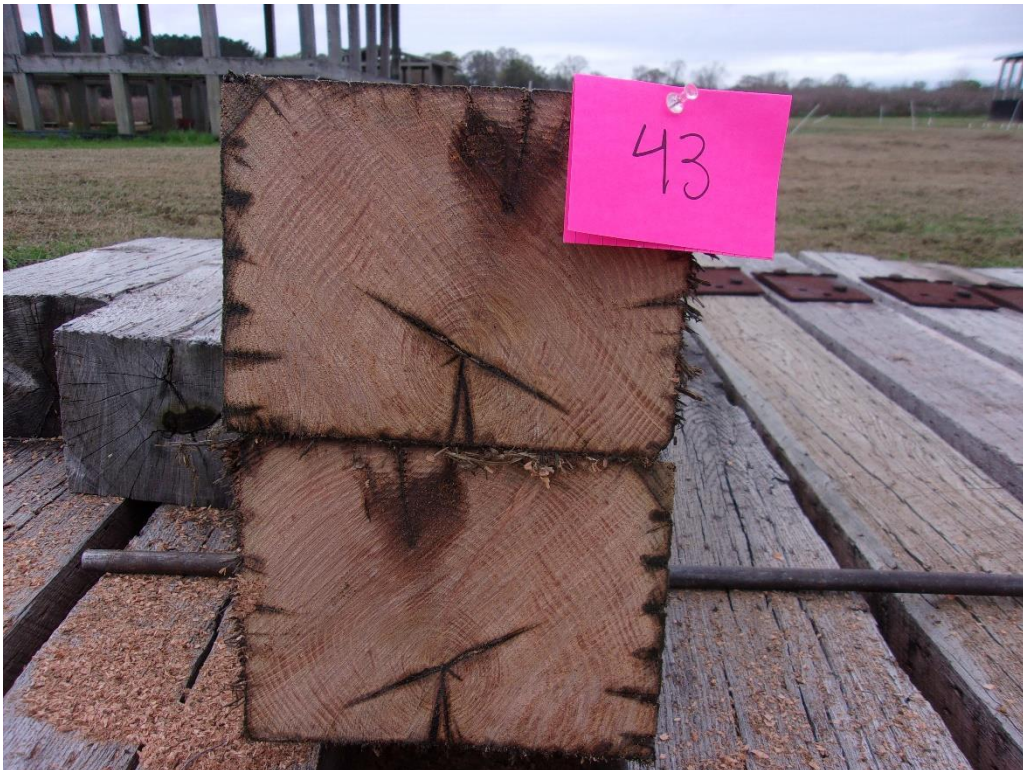
Figure 62 - Tie #43 white oak/DOT/ACZA/ET (Lonza).
