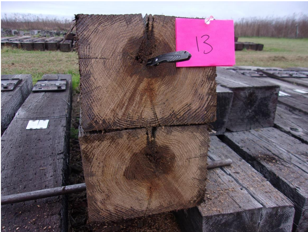
Figure 56 - Tie #13 red oak/one step creosote borate with decay in cross-section (Stella jones).
