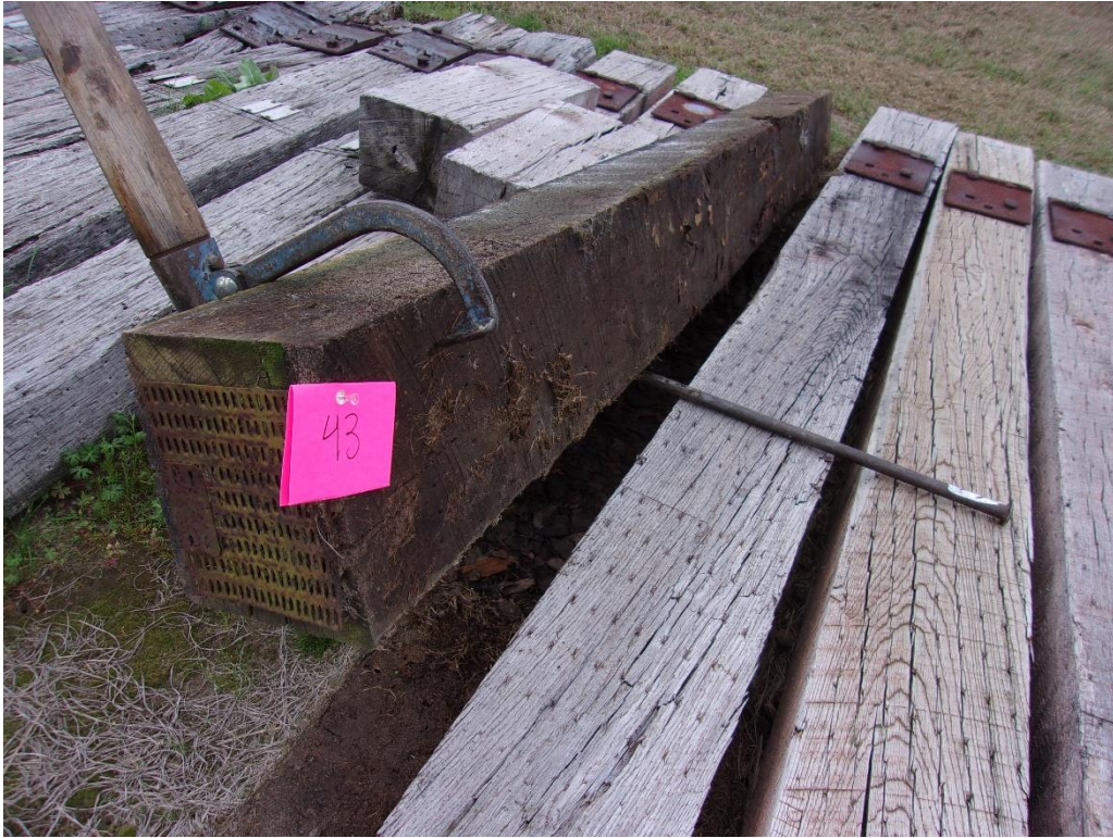
Figure 61 – Tie #43 white oak/DOT/ACZA/ET (Lonza).
