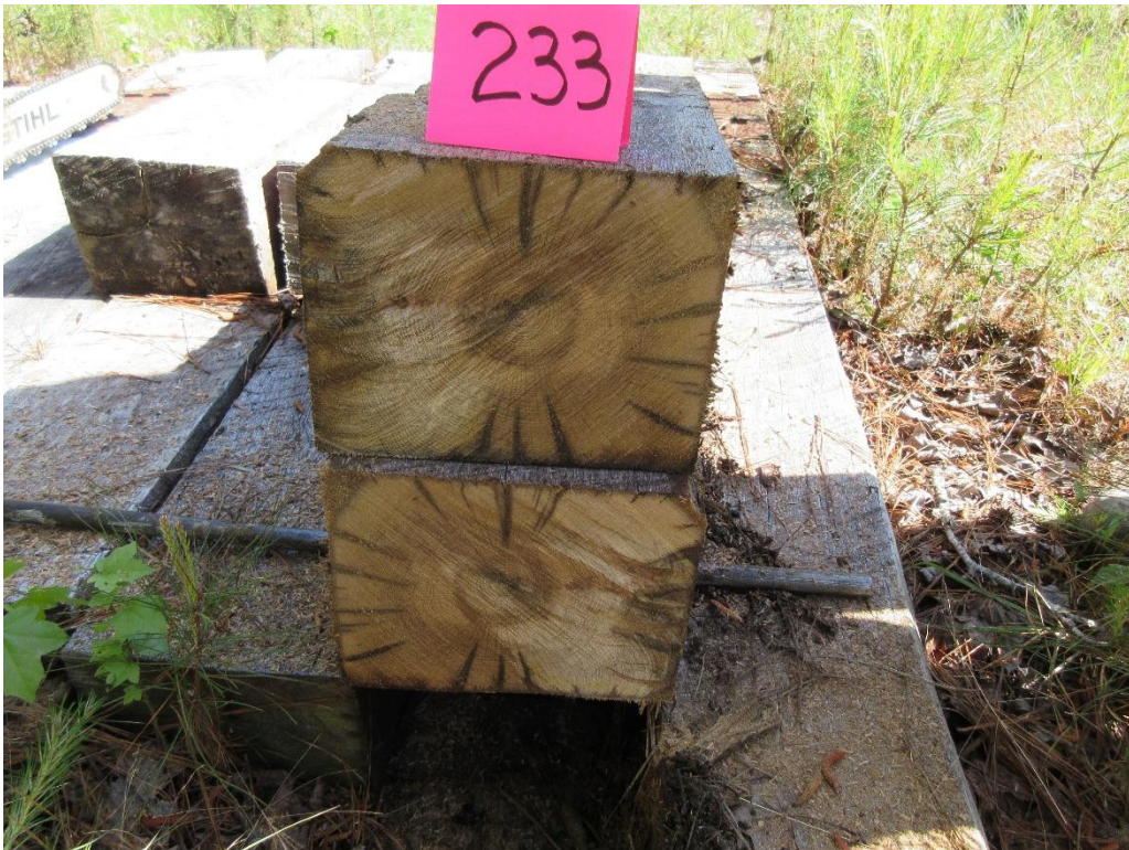
Figure 50 - Tie # 233 white oak/DOT/ACZA/ET (Lonza).
