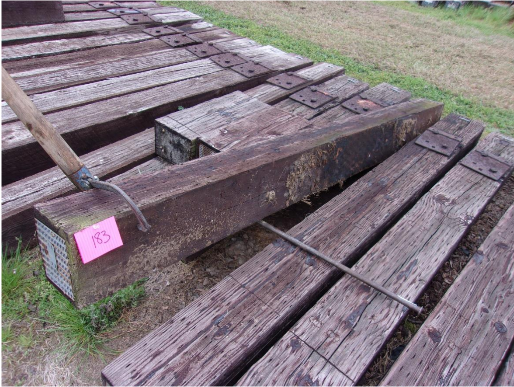
Figure 91 – Tie #183 Douglas fir/P2 (Lonza).
