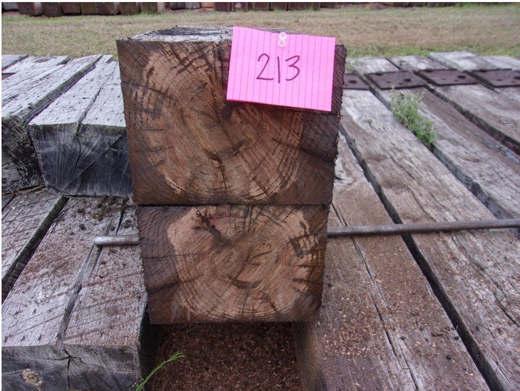
Figure 98 - Tie #213 red oak/borate/creosote 7lbs (Koppers).
