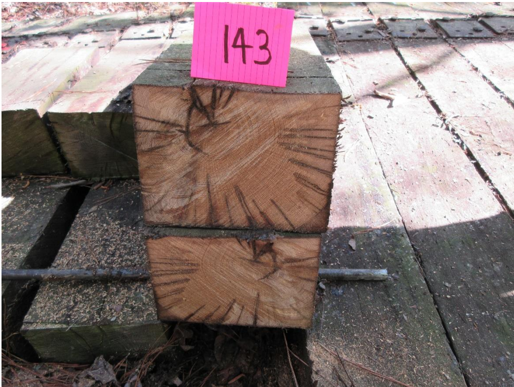
Figure 32 - Tie #143 white oak/DOT/ACZA/oil (Lonza).
