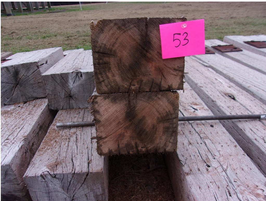
Figure 64 - Tie #53 red oak/DOT/ACZA/ET (Lonza).
