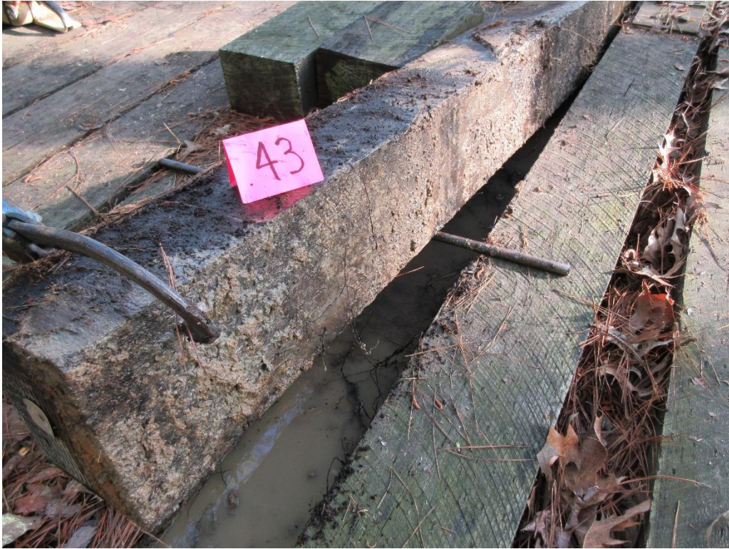
Figure 9 - Tie #43 white oak/borate/creosote 7lbs (Koppers).
