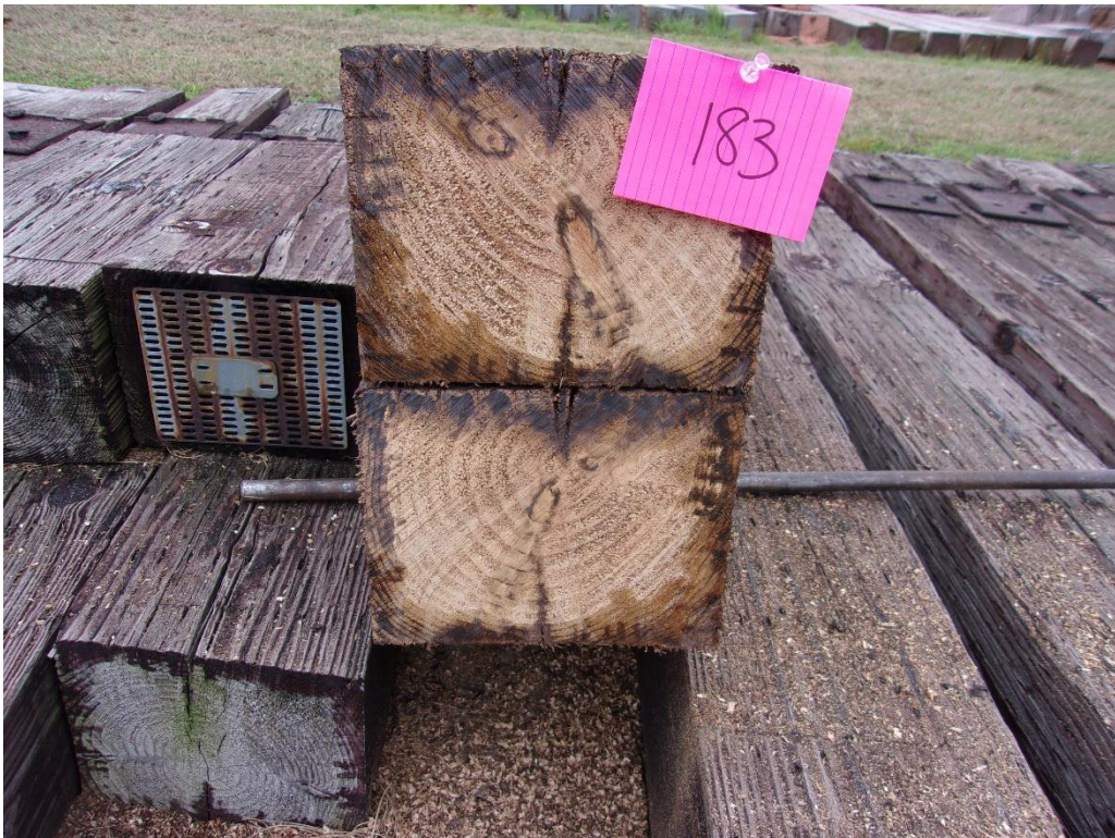
Figure 92 - Tie #183 Douglas fir/P2 (Lonza).
