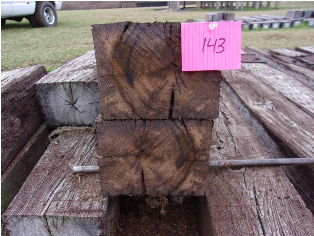
Figure 82 – Tie #143 red oak/DOT/ACZA/oil (Lonza).
