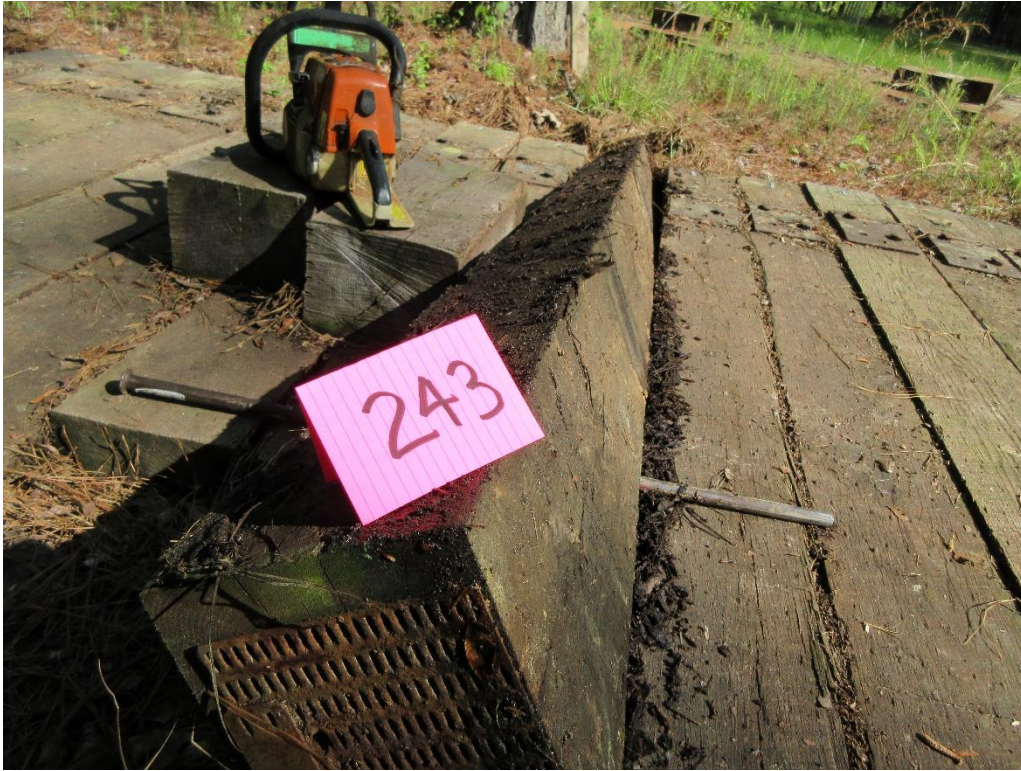
Figure 51 – Tie #243 red oak/ACZA/DOT/ET (Lonza).
