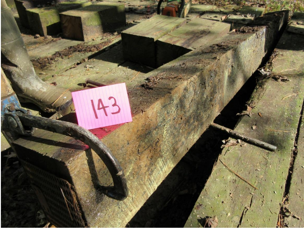
Figure 31 – Tie #143 white oak/DOT/ACZA/oil (Lonza).
