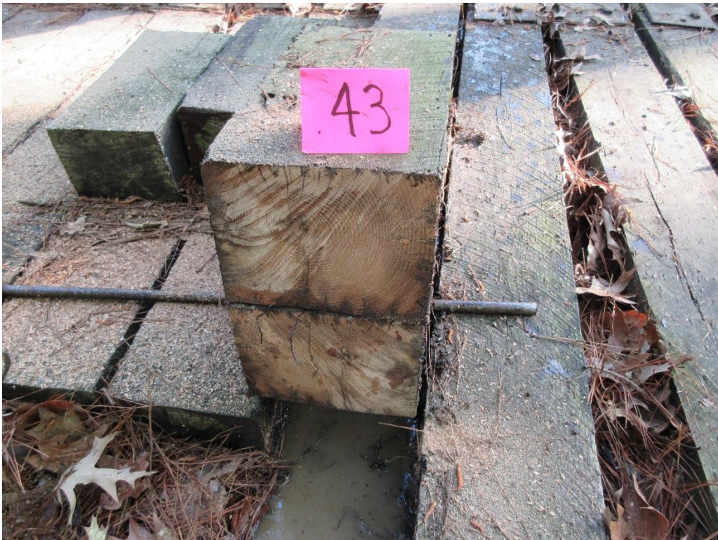
Figure 10 - Tie #43 white oak/borate/creosote 7lbs (Koppers).
