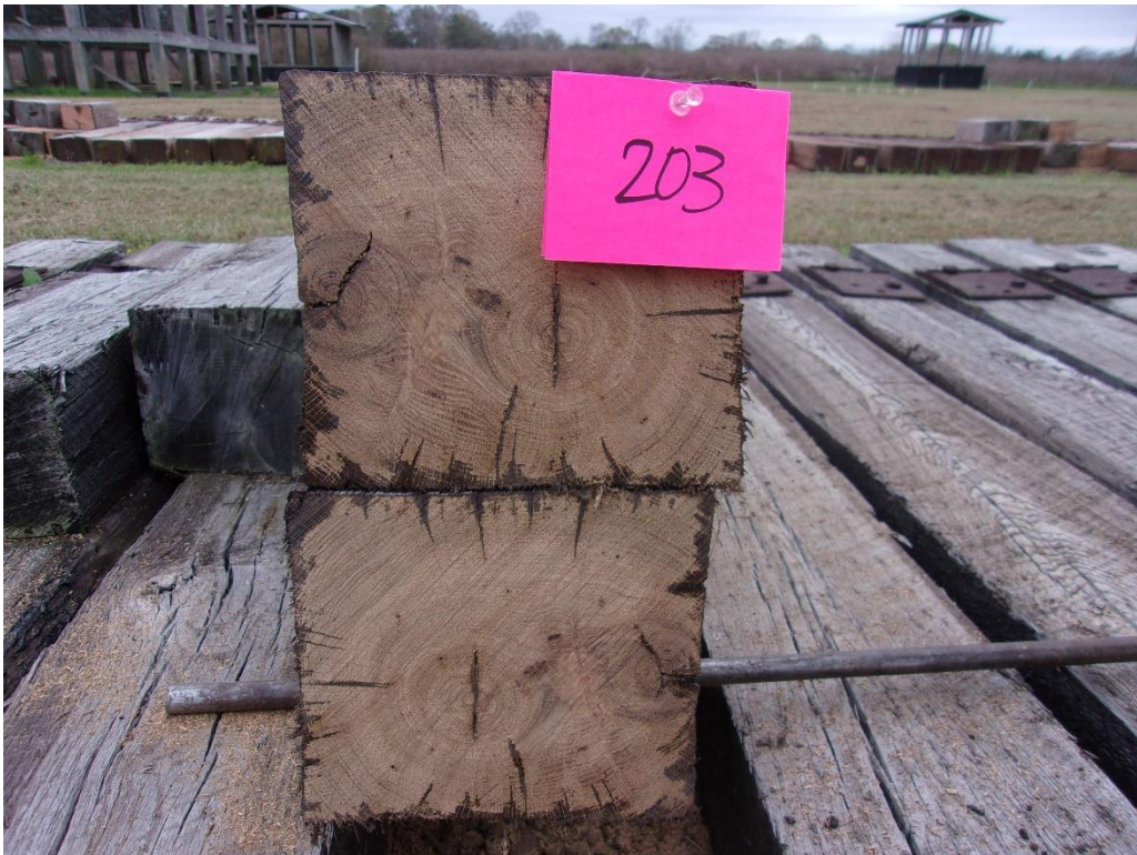
Figure 96 - Tie #203 white oak/borate/creosote 7lbs (Koppers).
