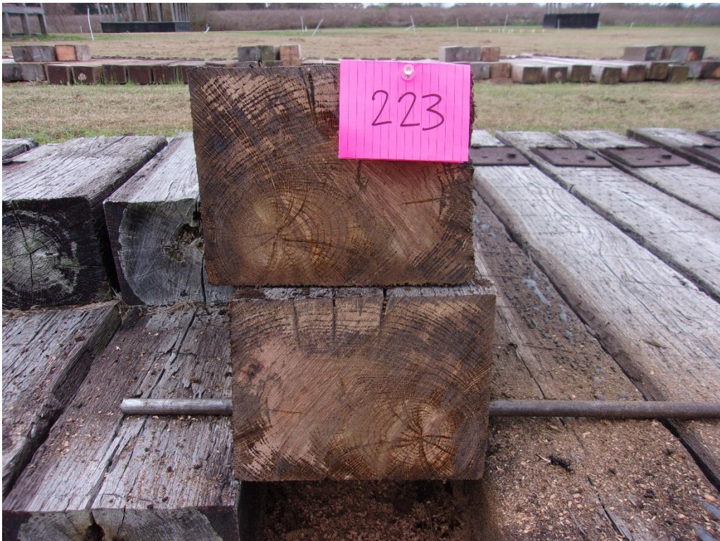
Figure 100 - Tie #223 red oak/borate/creosote 6lbs (Koppers).
