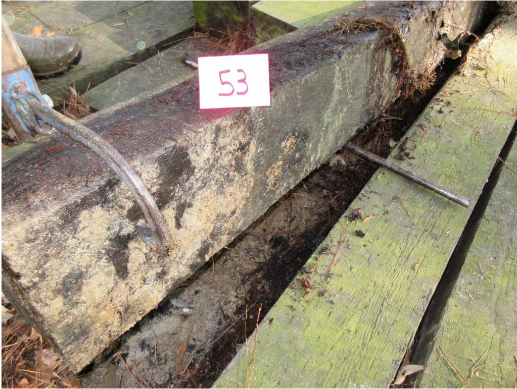
Figure 11 - Tie #53 red oak/borate/creosote 6lbs (Koppers).
