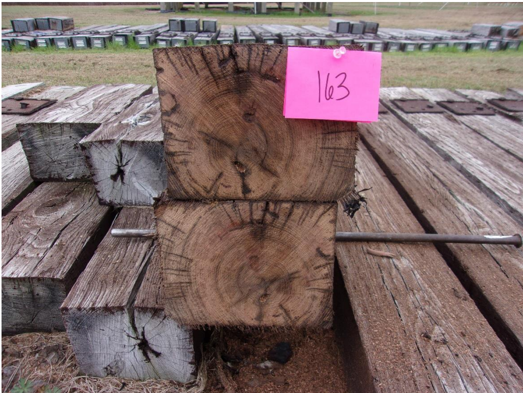
Figure 88 - Tie #163 red oak/DOT/ACZA/oil (Lonza).
