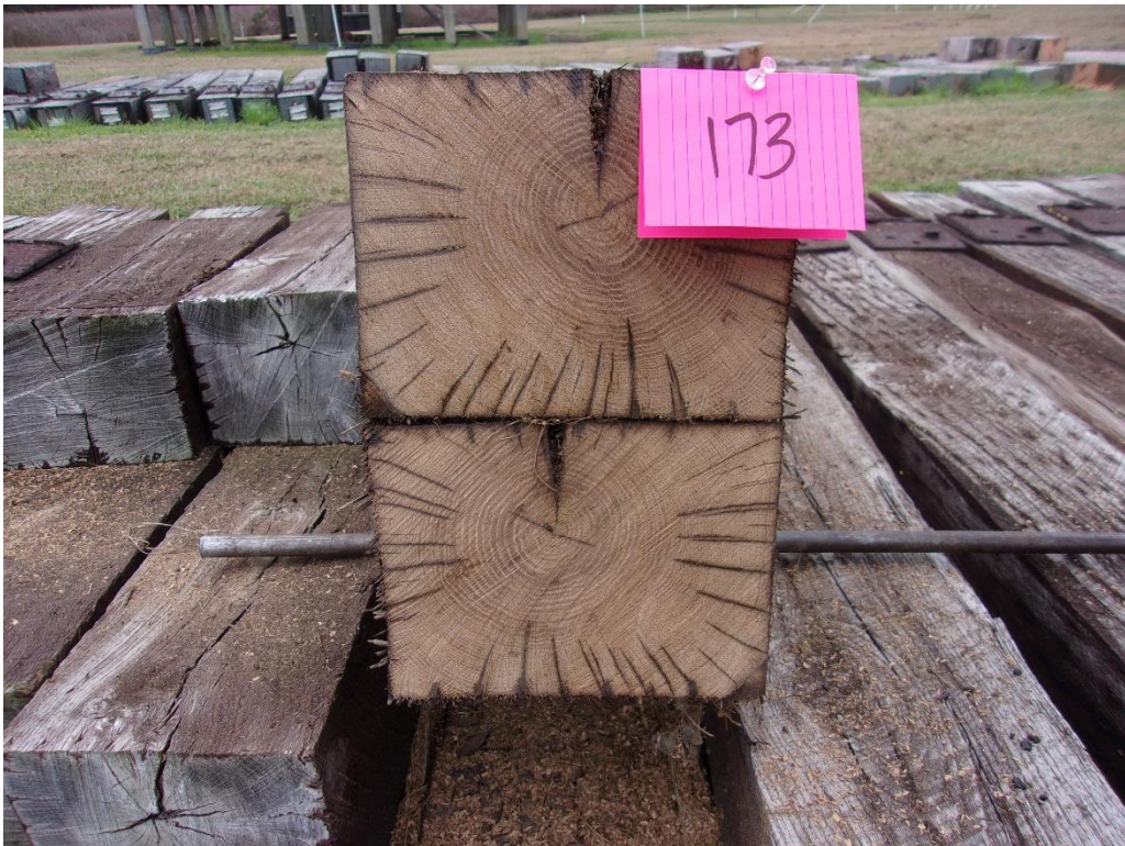
Figure 90 – Tie #173 white oak/DOT/ACZA/oil (Lonza).
