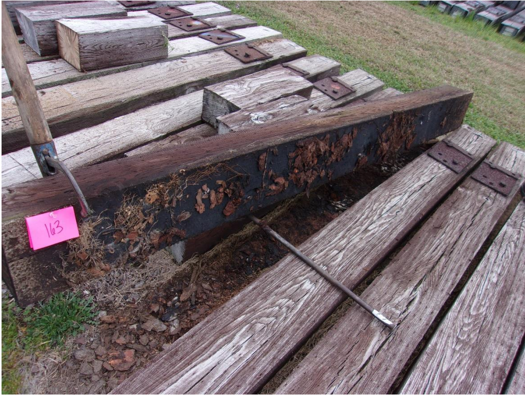
Figure 87 – Tie #163 red oak/DOT/ACZA/oil (Lonza).
