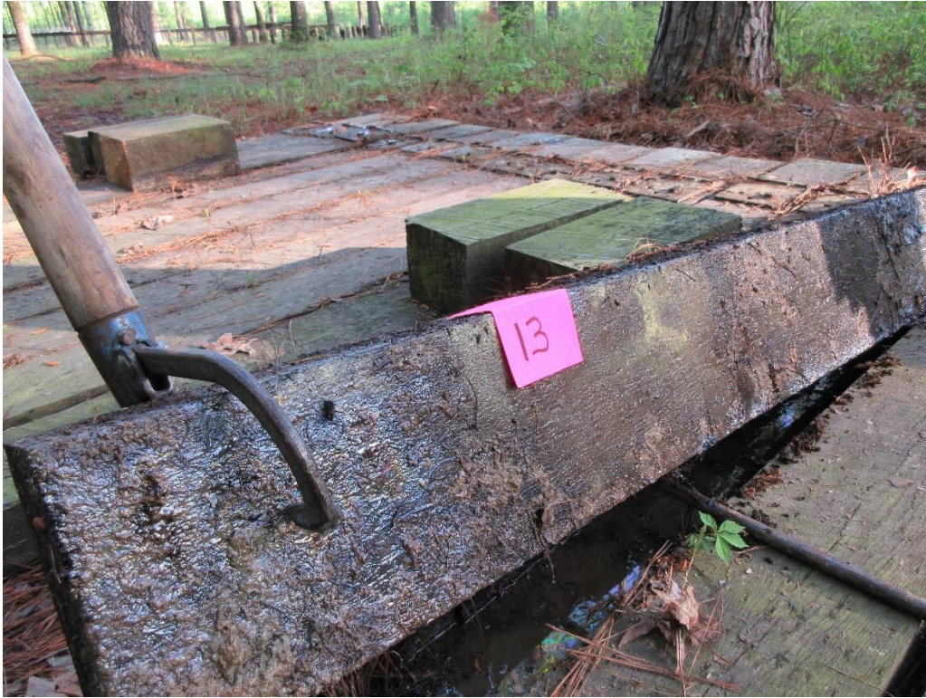
Figure 3 - Tie #13 red oak/borate/creosote 7lbs (Koppers).
