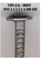
In other words, all the nails with the "P" under the head came from one manufacturer, in this case the Pittsburgh Steel Company. The ones with the "V" on the shank under the head were manufactured by the Republic Steel Corp.
