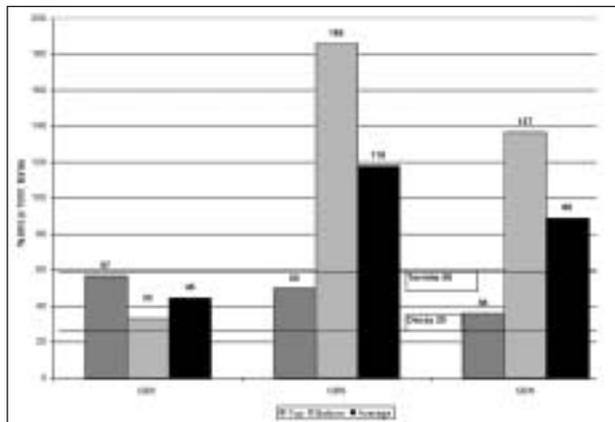
**Figure 1.** Borate analyses of borate-treated mixed hardwood (red and white oak, hickory and gum) ties over-treated with creosote by dip (GBC) or pressure GBS – Atchison, Topeka & Santa Fe treatment GBN – Norfolk-Southern treatment after 15 years of field exposure. Analysis zones were from the upper or lower tie surface to the center.
