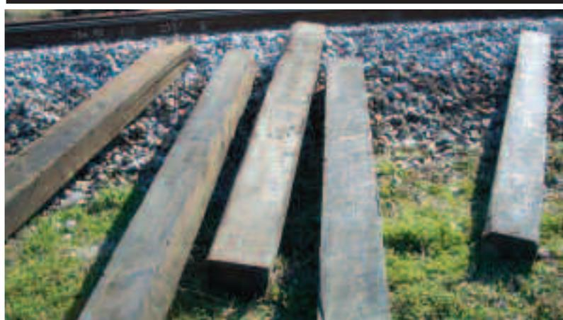
Research has proven that wood crossties pre-treated with borate, then over-treated with creosote, last longer in track, especially in the Southern United States.
