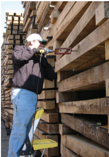
One quality control step is to measure retention/penetration of borates at various stages during processing.
