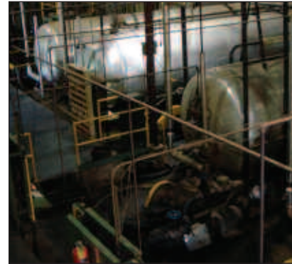
After that, the ties are restacked for air seasoning. Then, a few months later, they are treated with creosote (above). Jim Standish (right) discusses the process from the treating plant perspective.
