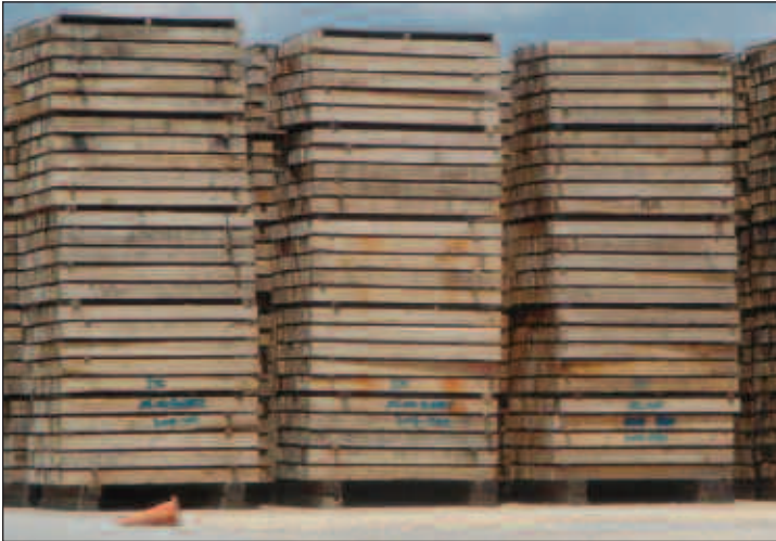
After that, the ties are restacked for air seasoning. Then, a few months later, they are treated with creosote (above). Jim Standish (right) discusses the process from the treating plant perspective.
