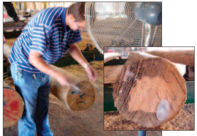
One of the requirements for all electric utility pole producers is branding and tagging each pole. Here, one of the tags identifies to whom this pole will be shipped.
