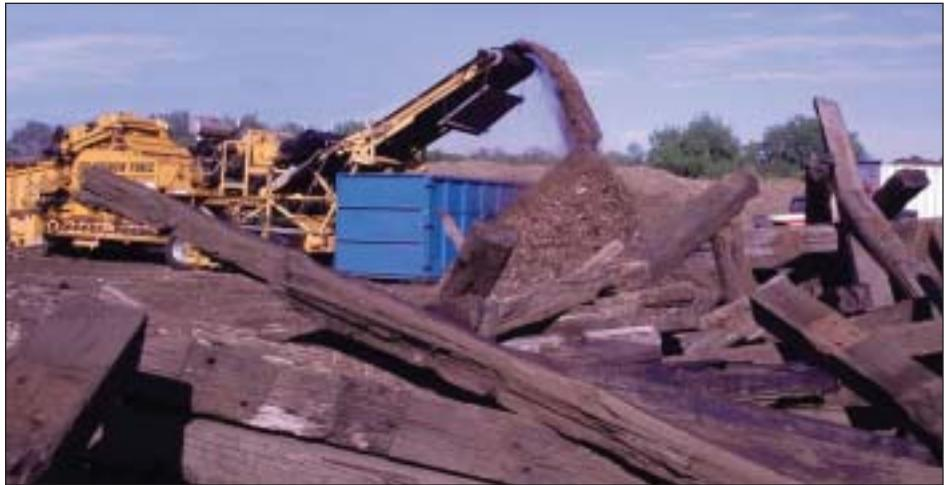
Between being picked up off a railroad's right-of-way and being converted into fuel, many ties are ground by machines such as Continental Biomass Industries' Magnum Force grinders, as shown above.
