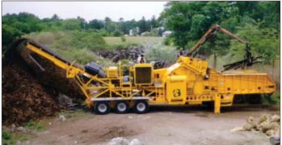
Continental Biomass Industries' Magnum Force grinders, such as the one shown above, help tie processing companies convert old railroad ties into usable material for cogeneration plants.
