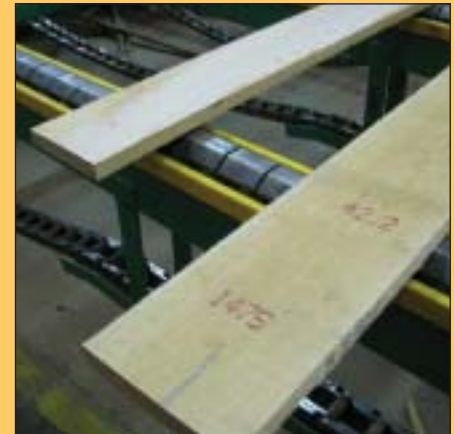
The computerized process can be set to spray identifying numbers on the boards so that sorters can efficiently pull exactly the right material for the customized orders.
