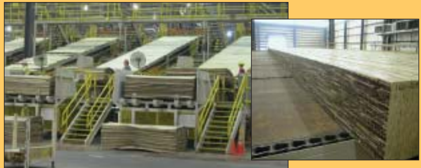
For Parallam, lower-grade veneers (those in which imperfections can be clipped out) ascend the production line to be clipped into smaller pieces before being reformed into major structural components like bridge timbers up to 66 feet long.
