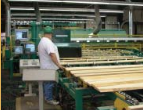
Just down the road from Armstrong, we made another impromptu visit to a Coastal Lumber facility. The company's Dailey Yard employs state-of-the-art computerization to sort and package grade lumber.
