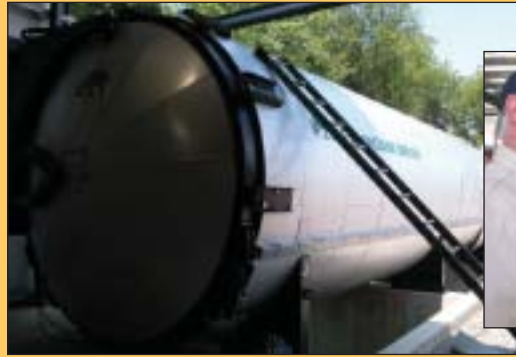
Marschat has also invested in a Danish-made vacuum dryer that can take 15,000 BF of 4/4 maple from green to dry in four days, eliminating the need for stain control chemicals that dull the wood.
