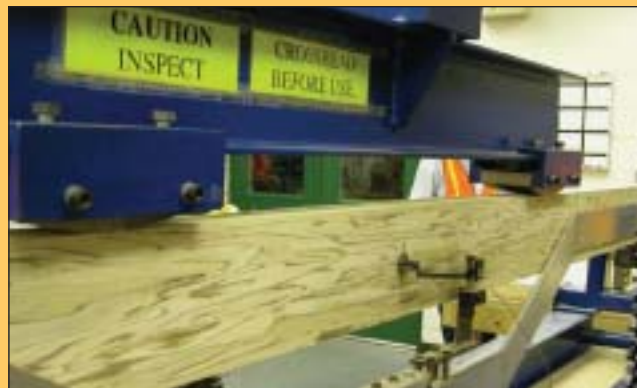
For Parallam, lower-grade veneers (those in which imperfections can be clipped out) ascend the production line to be clipped into smaller pieces before being reformed into major structural components like bridge timbers up to 66 feet long.
