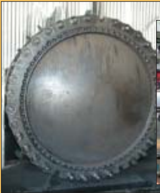
Old-styled bolted doors belie the sophisticated controls in use at the plant. The cylinders are all slated for replacement within the next few years.
