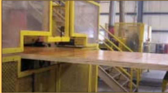
For Microllam, the veneers enter in whole pieces and emerge as a finished engineered product.
