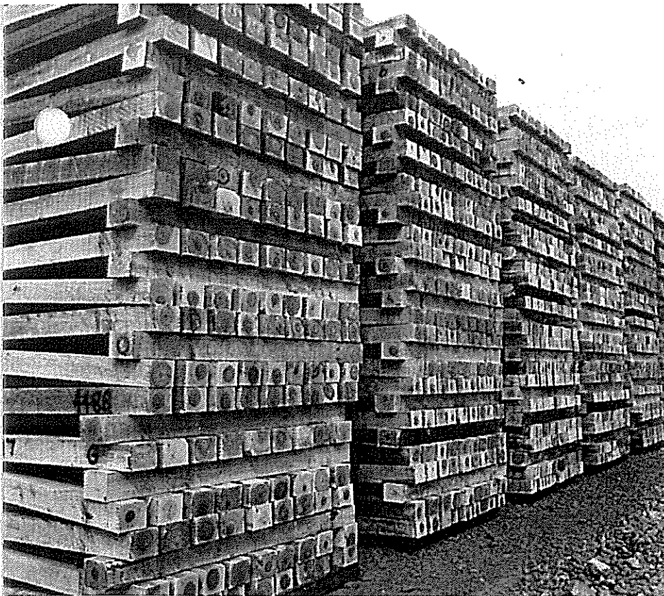
Depending on the wood species and drying conditions, wood crossties require four to 14 months of air seasoning. Stacking allows air to flow around each tie.
