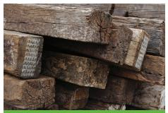
Storing used rail ties in the manner pictured above is not allowed in California. Hazardous waste should be stored, handled and transported under California regulations that prevent water runoff from the wood into the environment.
