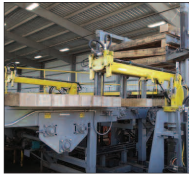
A superb incising operation and an automatic end plater that selectively end plates ties are stops along the way to the new automatic German stacker (installed in 2013) that stacks the ties for air-drying.
