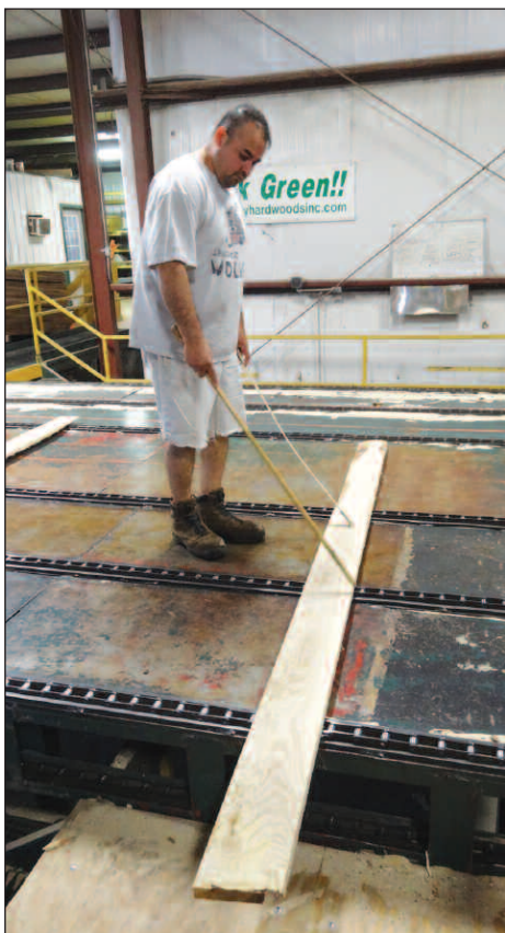
A lumber grader visually inspects and marks a board for grade and size.
