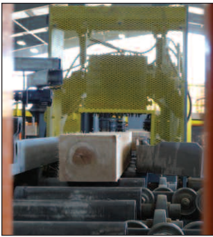
A superb incising operation and an automatic end plater that selectively end plates ties are stops along the way to the new automatic German stacker (installed in 2013) that stacks the ties for air-drying.
