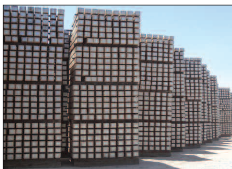
Here are some of the hundreds of thousands of ties air drying on the yard.
