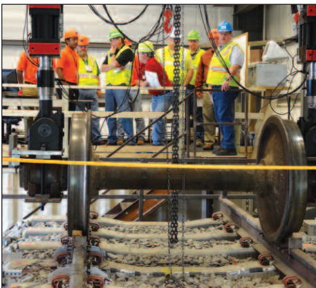
Day 3 starts with a tour of the Univ. of Illinois Urbana-Champaign where all attendees get to hear about the FRA-sponsored research conducted on the "to scale" test track bed. At the time, UIUC was testing a specific concrete tie and fastener configuration using a wheel set.
