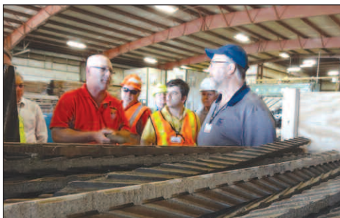
Boeding continues to illustrate how River City is merchandising high-end walnut and cherry for customers that require dried stock that have no sticker marks, these specialized grooved stickers do the trick.
