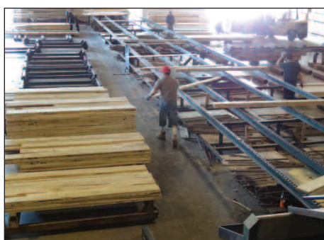
Then it is hand sorted by that size and graded along with any ties and timbers that come across the chain.
