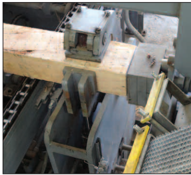
A superb incising operation and an automatic end plater that selectively end plates ties are stops along the way to the new automatic German stacker (installed in 2013) that stacks the ties for air-drying.
